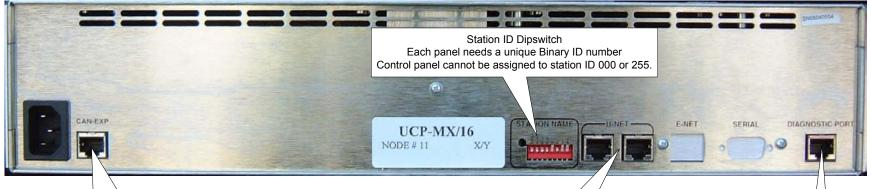
When an expansion panel is used, this connection loops between the panels using a CAT-5 cable. When no expansion panel is used terminate this connection with the supplied U-Net terminator.
